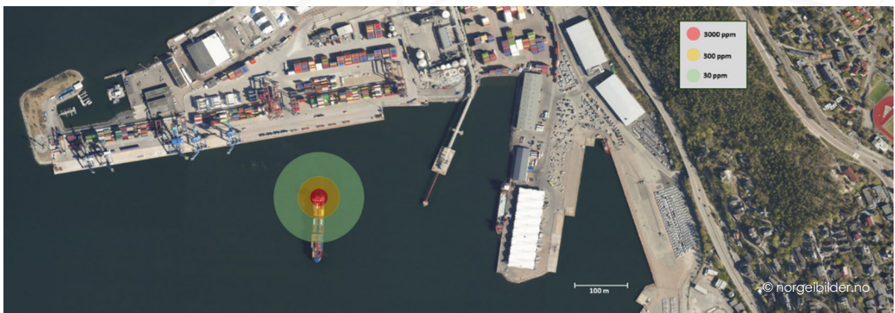
Figure 3 – Illustration for a dispersion contour for ammonia operation.
