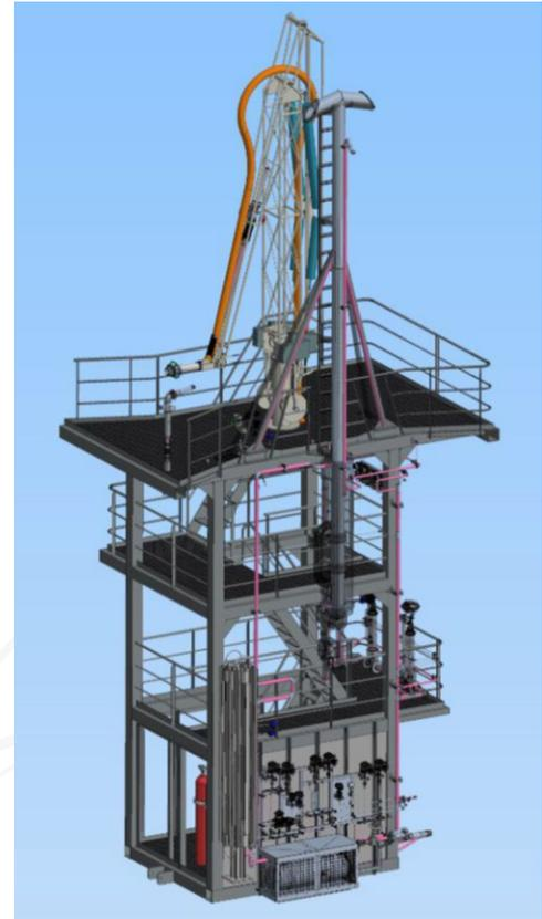
The equipment is installed on a skid, mounted on wheels, to ensure easy transportation to the quayside.
